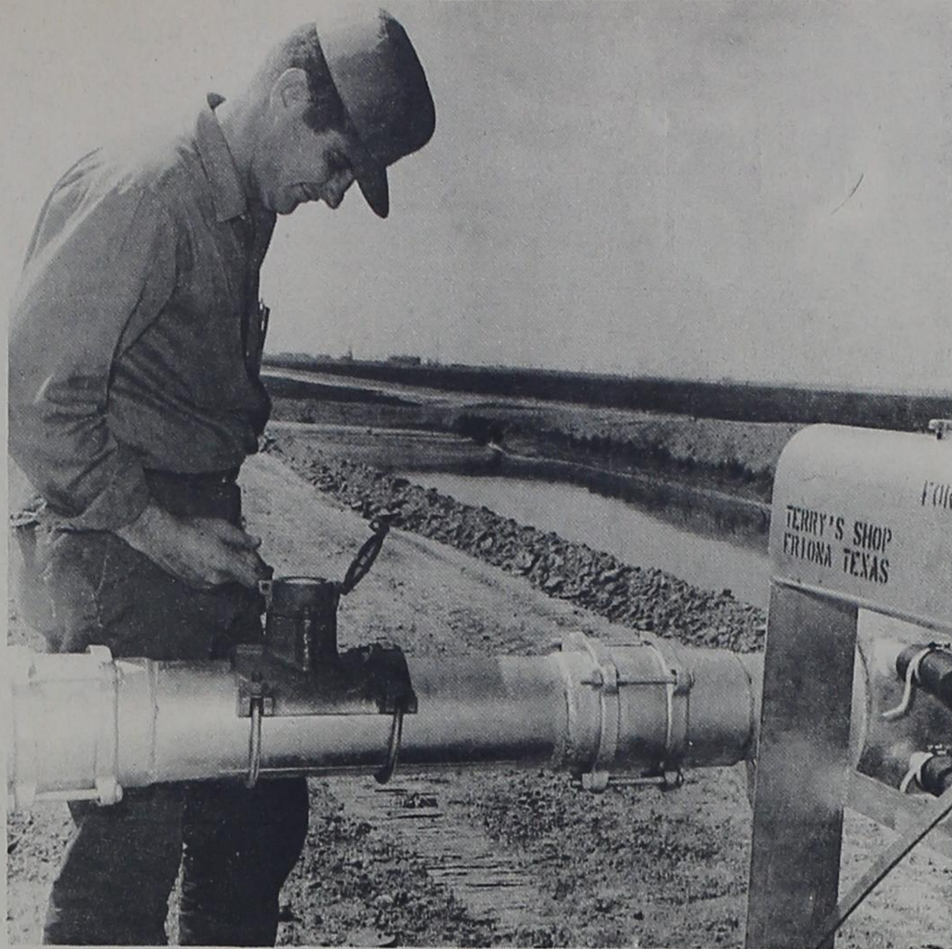
MAKING A READING from a "flow meter" attached to a tailwater pump on the J. B. Taylor farm south of Friona is Wayne Wyatt of the High Plains Water District. At the time the reading was made, the pump was putting out 800 gallons per minute or 48,000 gallons per hour. Some pumps in the area are logging up to 72,000 gallons per hour, at a nominal fuel cost.
