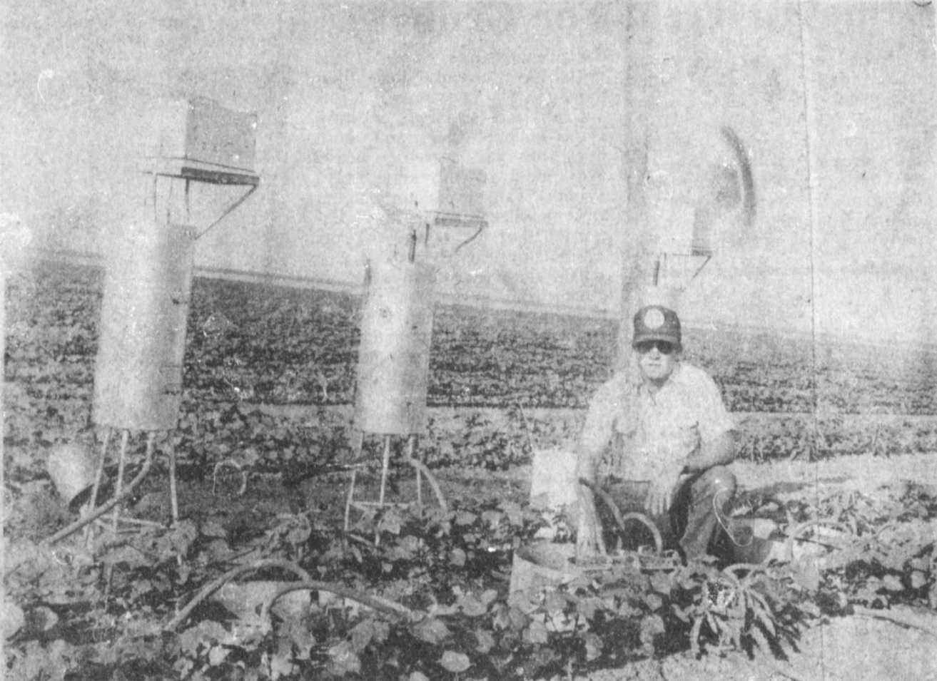
SOIL MOISTURE MONITOR TESTING—Warren Givens of the Blackwater Valley Soil and Water Conservation District is shown checking some of the equipment being used to monitor the absorption of moisture into soil on a farm to the south and west of Muleshoe. Plow pan density is affecting the rate of absorption, he explained, along with the amount of moisture being able to penetrate beyond the roots of the young crops.
