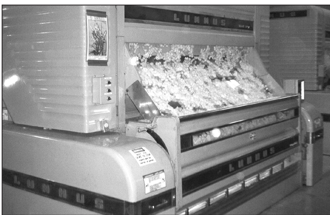
One of the machines that remove the burrs and seeds from the cotton.
