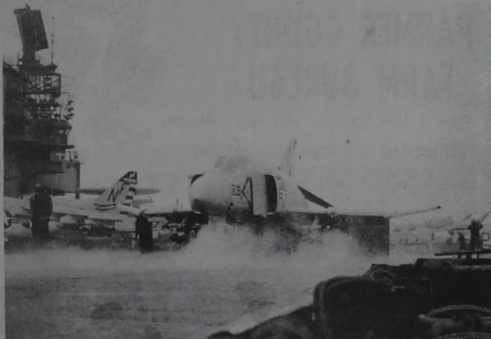
Steam escapes from the port catapult as an F-4 Phantom readies for launch from USS MIDWAY.
