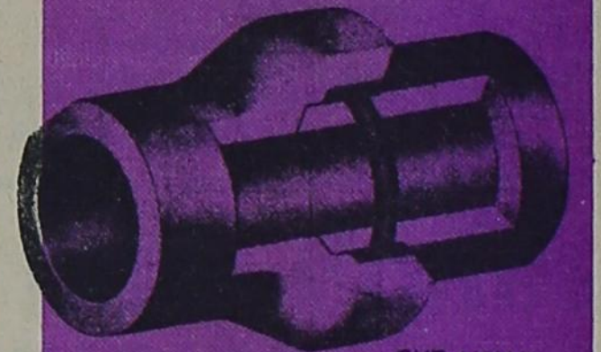
CUT-AWAY VIEW OF "O" RING SELF ALIGNING PIPE
