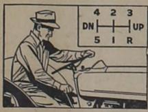
5-SPEED TRANSMISSION gives wide range of working speeds for best work, efficient engine operation.\*
