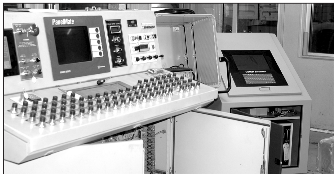
The control room received a new computer that judges color, trash and moisture and automatically updates with the Classing Office to look for possible variations.
