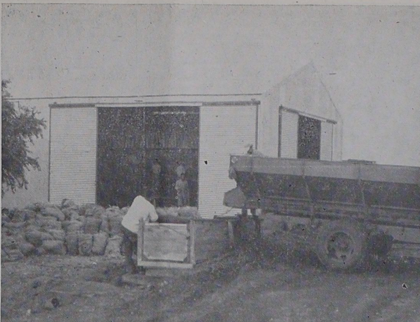
Special beds are used on trucks to bring potatoes in from the fields. Here a special conveyor carries the spuds out and dumps them into a waiting washing trough at the Gregory potato shed at Lariat.
