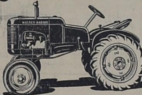
3-4-Plow 44—260-cubic-inch, 4-cylinder engine, 5 speeds forward.
