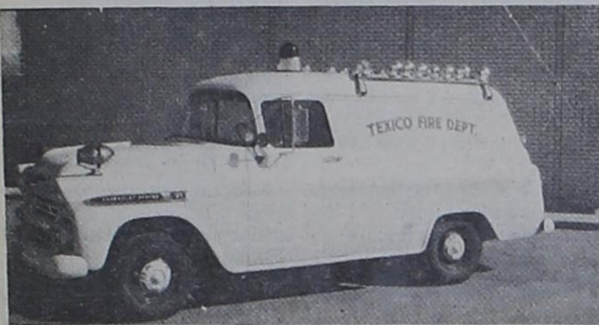
READY FOR SERVICE -- A half-ton panel truck is used by Texico Fire Department as an emergency vehicle. The van was overhauled and an eight-cylinder engine replaced a six-cylinder one. The Texico Fire Department pioneered the emergency vehicle service in this area.
