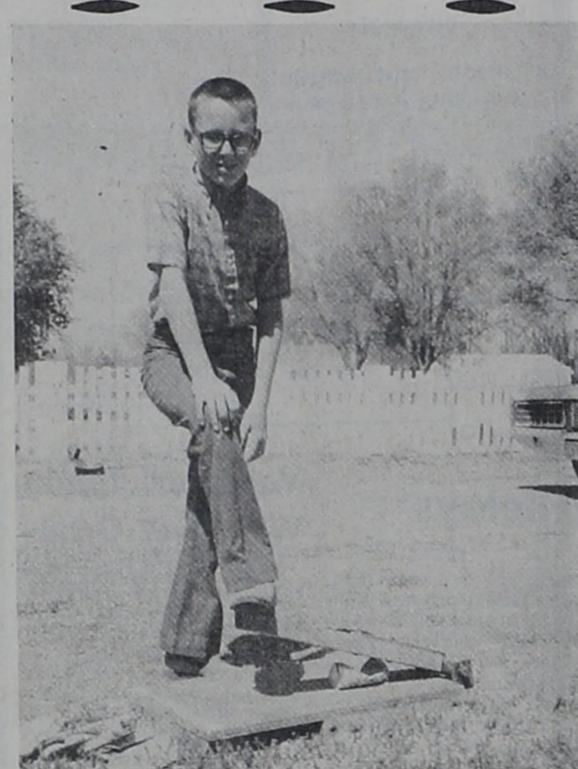
SQUASHING INVENTION -- Dwayne Obenshain liked the idea of squashing beer cans for recycling when he was looking for an individual money-making project to finance his Alaskan trip, but he figured there had to be an easier way than stomping, hammering or driving over the cans. He and his father collaborated on this squashing device using a board frame attached to a thick board lever by a large hinge fashioned from scrap metal. The lever can be operated either by hand or by foot.
