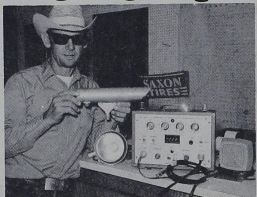
NEW FANGLED STOP WATCH -- This electronic timing device, demonstrated by Markum Chadwick, will be used to time contestants in each event of the AJRA rodeo. The device, which cost approximately $800, can measure the time it takes a contestant to complete an event or it can measure the amount of time which each contestant is given to complete a particular event. Both ways of measuring time will eliminate human error.
