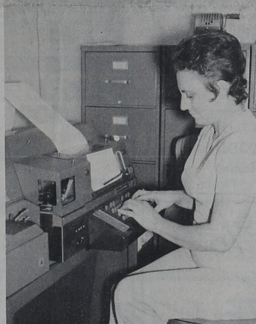
SHERIFF'S DEPARTMENT HELPERS—Mrs. Irene Woods operates the newly-installed teletype machine at the Parmer County Sheriff's office. The teletype, obtained through Panhandle Regional Planning Commission and furnished by Law Enforcement Assistance Administration, can obtain several types of information through a central computer in Austin while receiving messages from stations throughout the state.
