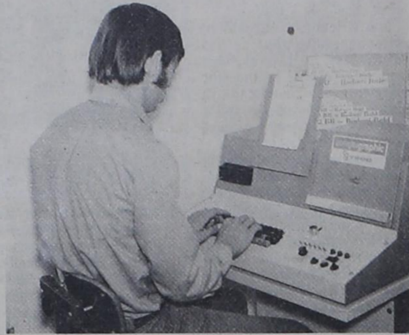
ASSORTED HEADLINES can be produced by this computerized headline machine which runs on the same principle as the typesetting machine. The headliner machine has a keyboard which allows the operator to make very small to extra large headlines with only a few adjustments. Ron Devenport, employee, finds it quick and easy to set headline copy.
