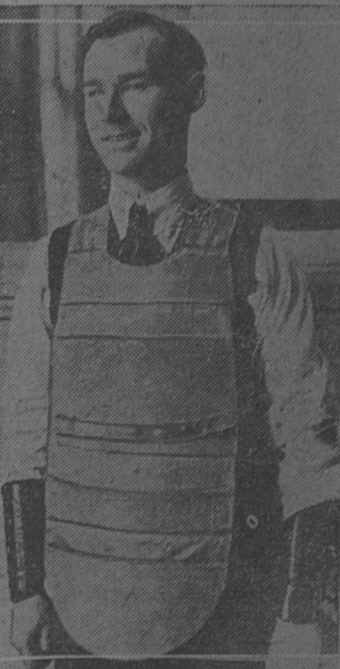
OMAHA COPS USE THEM —Special suits of light armor, capable of resisting steel-jacketed bullets of .45 calibre, are being used by the police of Omaha, Nebraska. The suit, composed of steel weights but eight pounds, will not interfere with the work of the officer.
