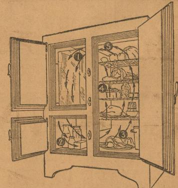
Here's where the warmest air in 1. the refrigerator enters the ice chamber and is rechilled and purified by contact with the five exposed sides of the block of ice. When you cover the ice, or put foods in the ice chamber, you interfere with the purifying and chilling of the air.
