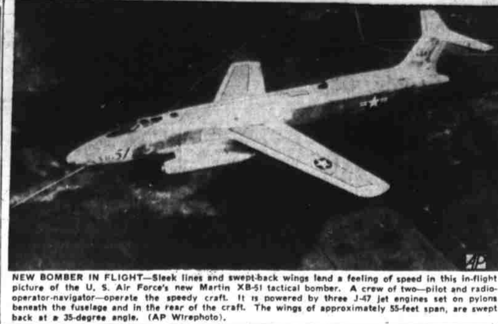
NEW BOMBER IN FLIGHT —Sleek lines and swept-back wings lend a feeling of speed in this in-flight picture of the U. S. Air Force's new Martin XB-51 tactical bomber. A crew of two—pilot and radio-operator—operate the speedy craft. It is powered by three J-47 jet engines set on pylons beneath the fuselage and in the rear of the craft. The wings of approximately 55-feet span, are swept back at a 35-degree angle. (AP Wirephoto).
