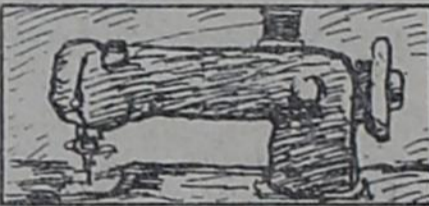
It took about 24 seconds on the earliest sewing machines to sew a hundred stitches.
