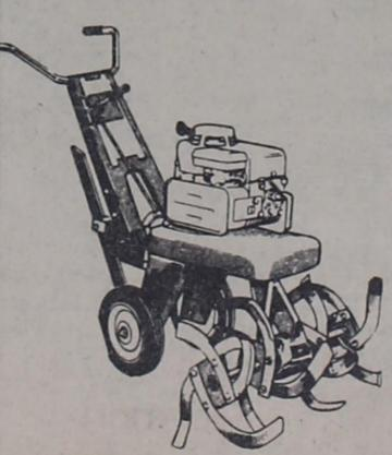
5 H.P. Briggs & Stratton engine. 26 inch width--14" diameter tines--forward, neutral, reverse--rewind starter--10"x 2.50 semipneumatic tires
