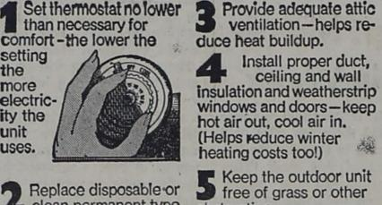
Replace disposable or clean permanent type obstruction a filters as required-clogged filters make the unit work harder anduse
