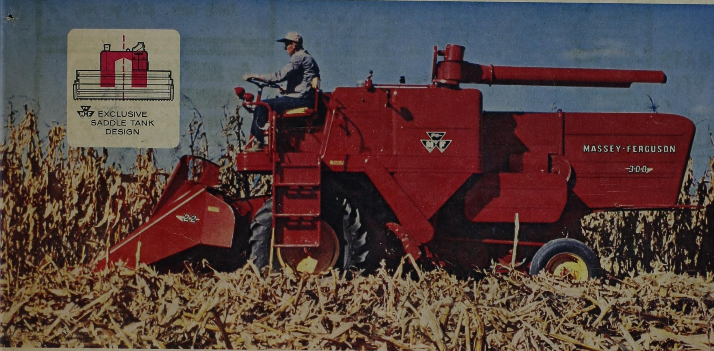
Massey-Ferguson 72 PT 8 or 10 ft. cut. 30 bushel grain tank. PTO or engine drive.
