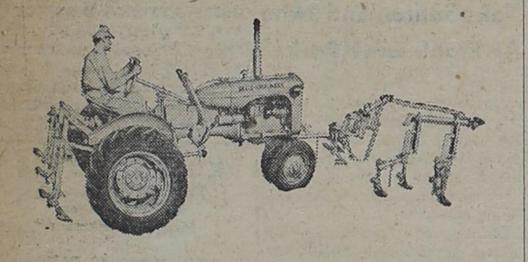
That's the way you mount Allis-Chalmers cultivators for CA, WD, and WD-45 Tractors. Gangs hinge open like a gate. You drive in, swing shut the gangs, and bolt them in place.
