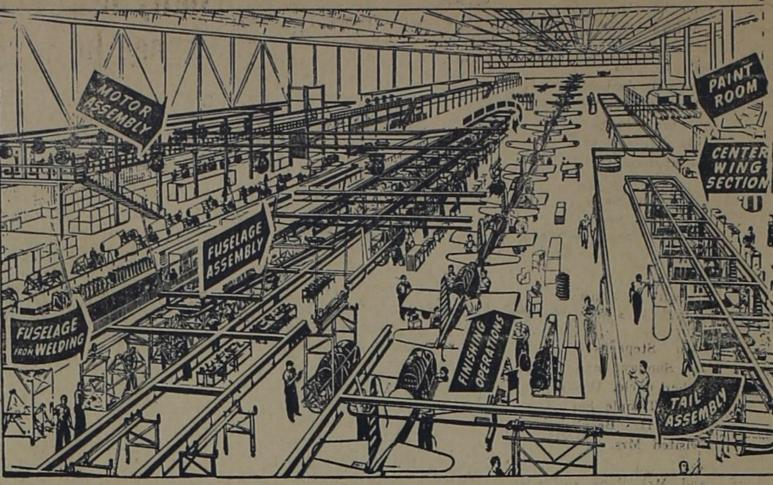
bly line shows the revolutionary production developments at the California plant in the last few months. It is the graphic story of how modern airplanes are with monocoque, stabilizers, rud- chain-driven overhead conveyor made compared to the methods of ders, elevators and control cables, but a year or two ago, and shows and move around on tracks to the the first mechanized assembly line center. Meanwhile, at the left, in the aircraft industry.
