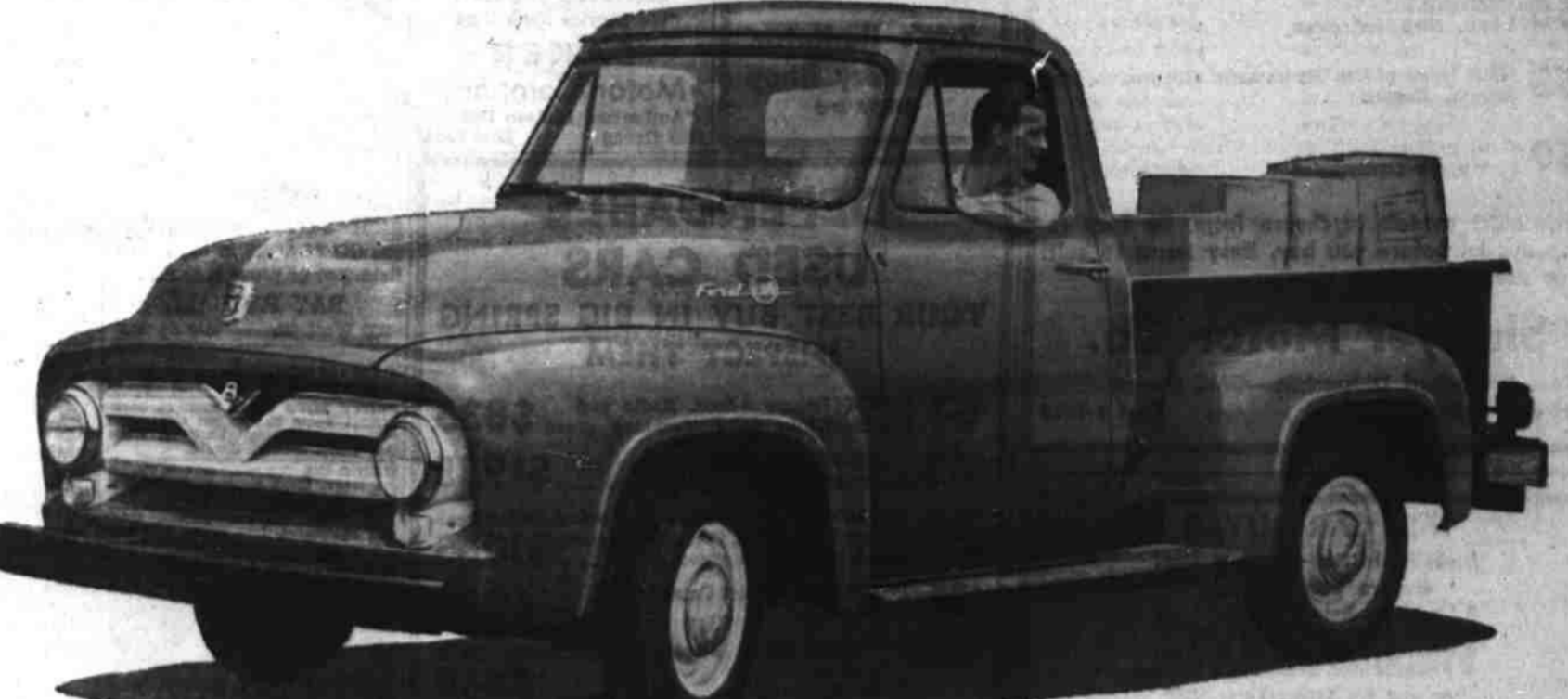
Ford 6 1/2-ft. Pickup gives choice of Short Stroke 132-h.p. V-8 or Short Stroke 118-h.p. Six. Tubeless tires standard. Fordomatic Drive and Power Brakes available at low extra cost. GVW 5,000 lbs.
