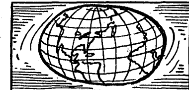
The earth is not perfectly round. Distances measured through the poles are shorter than those at the equator.
