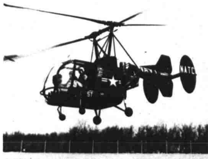
The world's first twin-turborotor helicopter, a joint Army-Navy project, flies with one or both of its 190-horsepower engines operating. Photo was taken during its first flight.
