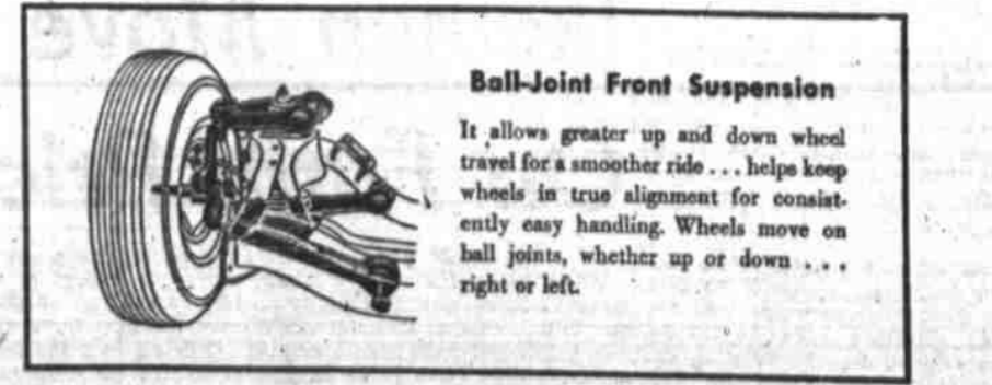
Ball-Joint Front Suspension It allows greater up and down wheel travel for a smoother ride... helps keep wheels in true alignment for consistently easy handling. Wheels move on ball joints, whether up or down... right or left.
