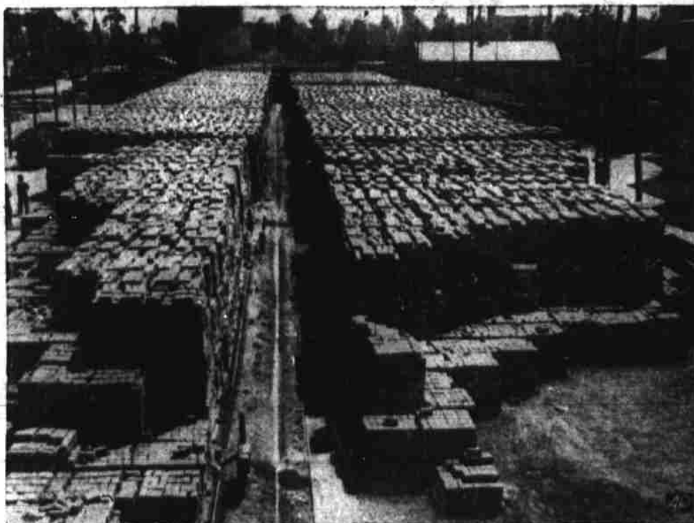
MODERN TRANSFORMATION —Bricks processed from rubble await shipment from a factory at Frankfurt-on-Main, Germany, for use in reconstruction of the war-damaged city.
