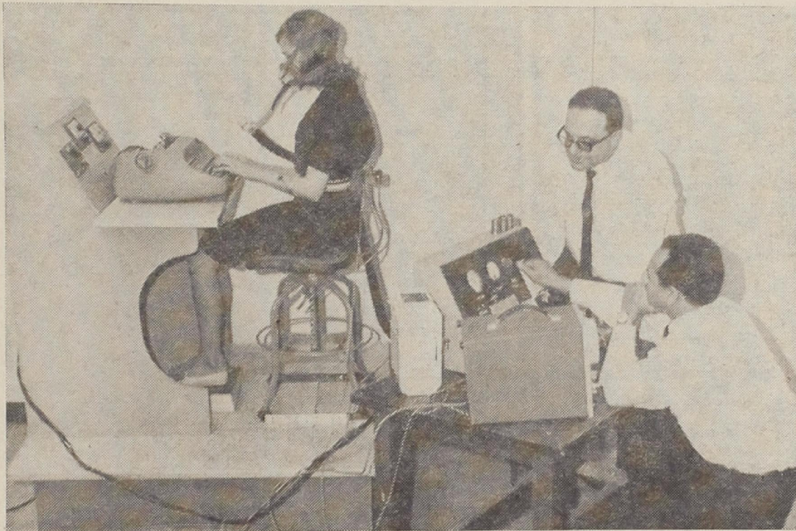
VIBRATION VERSUS MOTION — Texas Tech's Dr. Erwin Tichauer, center, and Dr. M. H. Ayoub investigate influence of verticle vibration on performance of fine hand motions in research project in Tech's Department of Industrial Engineering.
