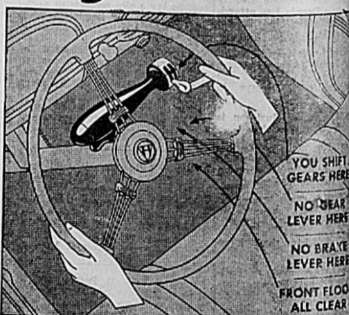
The Electric Hand, an optional extra, is mounted conveniently under the steering wheel.
