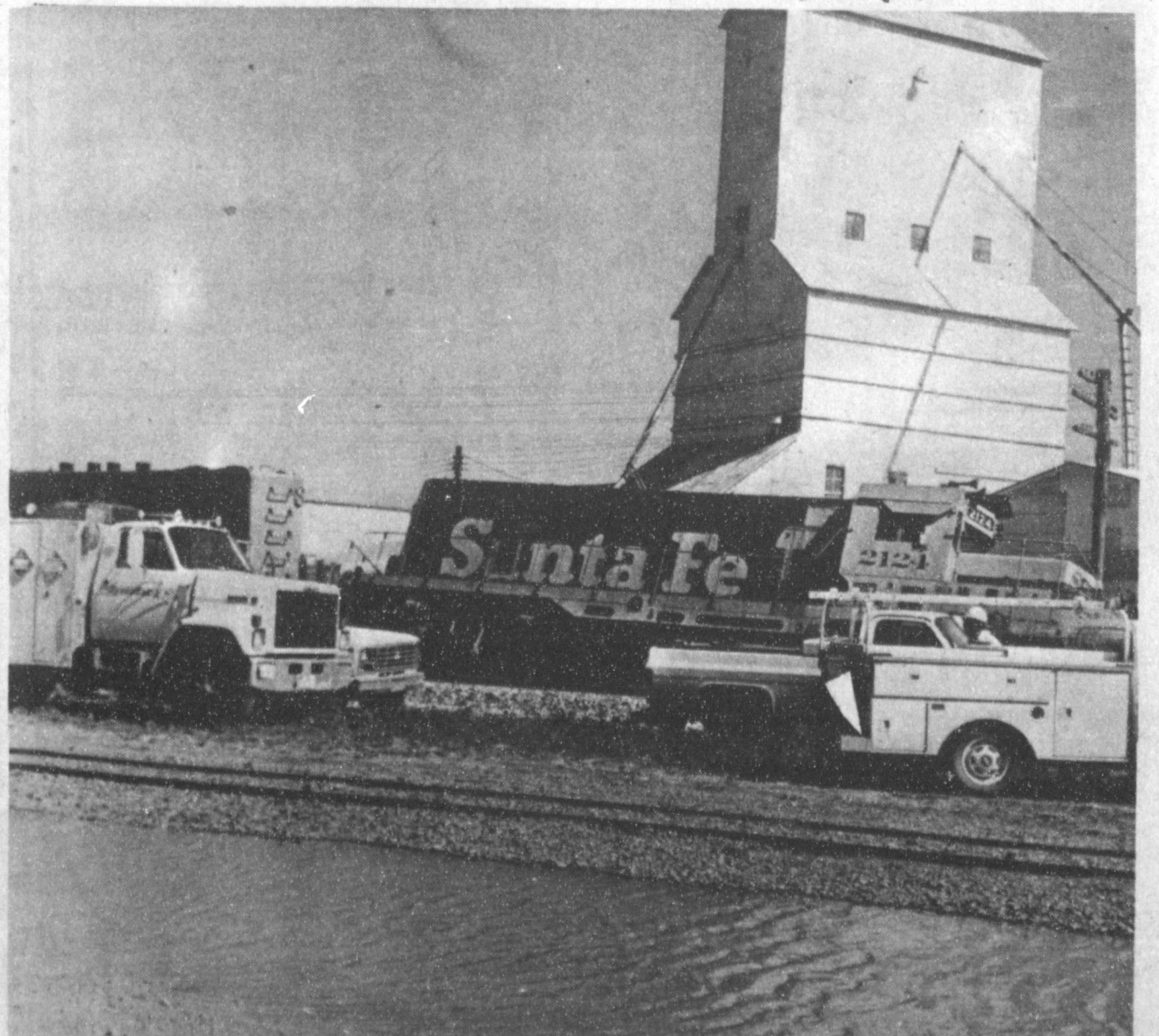
MINOR DERAILMENT FRIDAY MORNING --This engine from a Santa Fe train is shown leaning precariously in Muleshoe Friday morning. Between 9:15 and 9:30 on Friday morning, the engine was derailed just west of John's Custom Mill on East American Blvd. A spokesman for Santa Fe from Lubbock said the recent rains caused a 'rail spit' which caused the engine to topple off the track. No injuries were reported and train traffic was not stopped as the derailment was on a side track.
