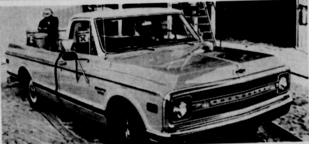
A 1.6-inch wider rear tread and 15-inch bias belted ply tires are among many improvements in the 1970 Chevrolet half-ton pickup. Side marker lights and reflectors are standard, and all engines are equipped with a new type exhaust emission control system. New options include sliding rear window, 400-cu.-in. V8, air-inflatable rear shock absorbers with coil springs to maintain a level ride with varying loads, and a tilt steering wheel with automatic or 4-speed transmission.
