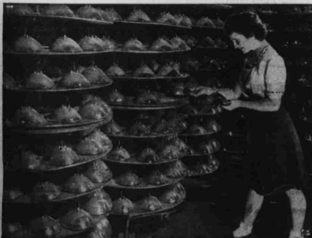
LANDING LIGHT 'MIRRORS' — Glass reflectors for sealed beam landing lights in military aircraft are placed on racks by a girl worker in the Westinghouse plant at Bloomfield, N. J.
