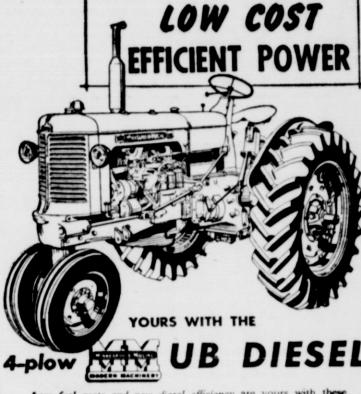
Minneapolis-Moline UB diesel features . . . Lanova combustion system provides rotary-turbulence action for a smooth and even, powerful piston stroke. Three-stage filter cleans fuel thoroughly before it enters the injection pump, gives you trouble-free performance. Single-plunger fuel pump feeds an accurate, evenly measured amount of fuel to the combustion chamber, gives you
