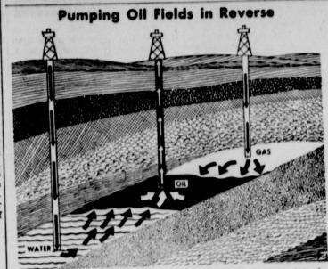
PITTSBURGH, PA.—By pumping water and natural gas into the depths of the oil fields, modern science is bring 10 to 50 per cent more oil to the surface. This typical cross section shows one way it's done. Here gas is pumped in above the oil pool, and water underneath it. These artificial pressures, from above and below, force the oil to flow thru the sand or rock in which it is imbedded and up the well shaft. Sketch is based on an explanation by Gulf Oil.
