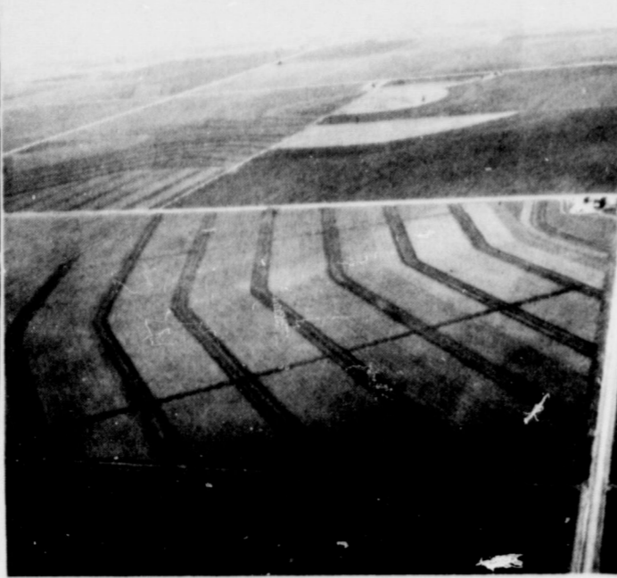
NEW system of parallel terraces cost shared under GPCP, designed and laid out by LaMesa Soil Conservation
