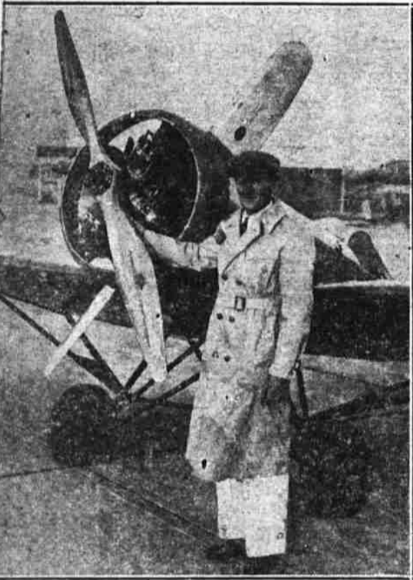
Charles L. Brown, gasoline dealer at Rushville, Mo., offers this idea tandem propellers, revolving in opposite directions, as a means of overcoming airplane "torque"—the tendency of a plane to be pulled off its course by its propeller. (Associated Press Photo)
