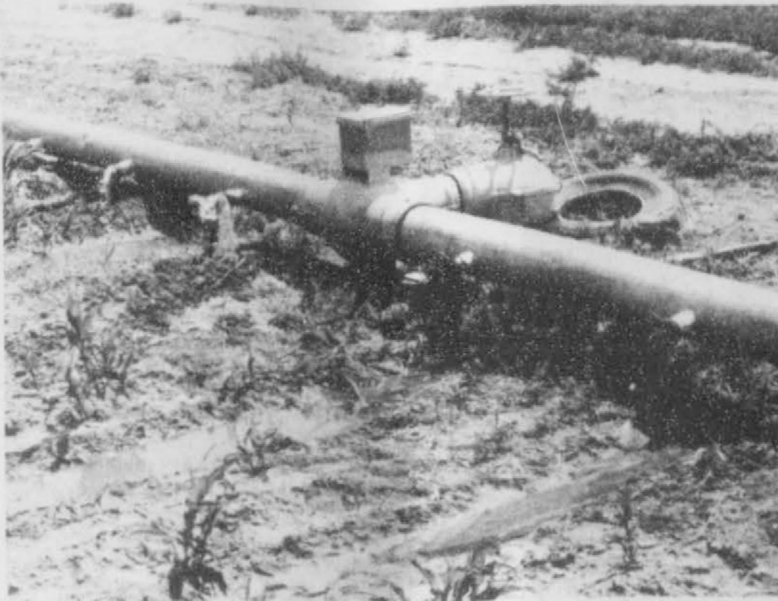
Surge Valve being utilized to save: pumping energy, labor and time.
