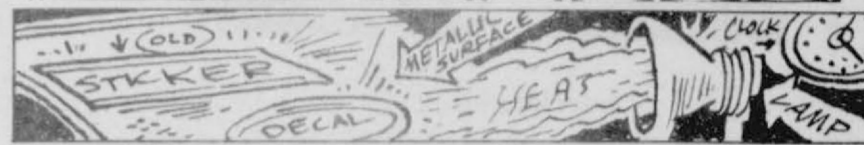
To remove old stickers and decals from metallic surfaces, place a heat lamp over the decal for five to ten minutes.
