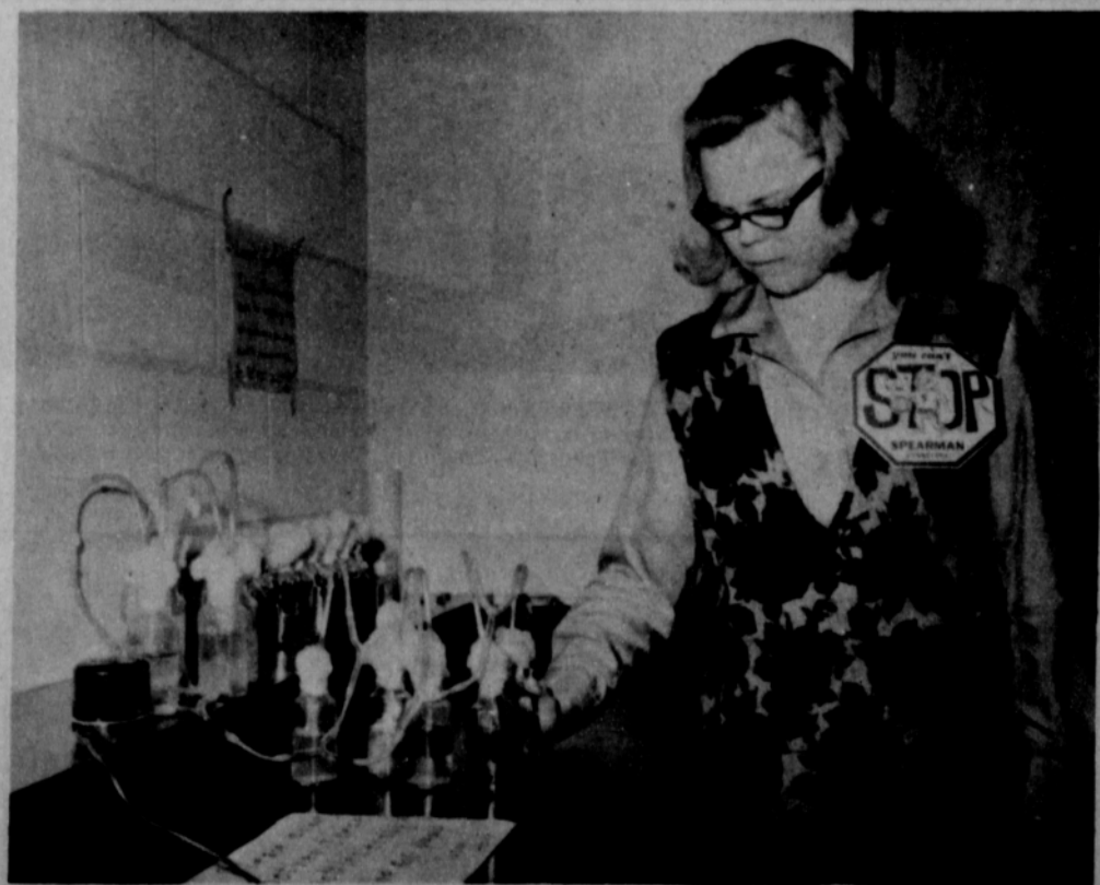
FUEL EXPERIMENT - Susan Holt is conducting an experiment on micro-organisms in fuels. The micro-organisms live on carbohydrates from the fuel and inorganic salts from the metals. They damage fuel tanks in aircraft and are a major problem. Plainsman photo
