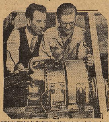
What is claimed to be the lightest airplane motor ever built, developing 450 horsepower, is the invention of Kenneth W. Barkman, left, and N. E. Cherdavoine of Los Angeles. The engine is a semi-turbine rotary AB HOA type, one-sixth the size of an ordinary motor. It has no pistons, cams, sleeves or valves, is built in two housings with 15 parts, and because of its simple construction is said to encounter practically no friction in operation. It weight only 220 pounds.
