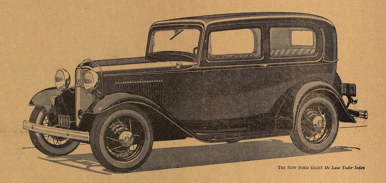
Eight-cylinder, 90-degree V-type, 65-horse-power Engine \* Vibrationless Roomy, Beautiful Bodies \* Low Center of Gravity \* Silent Second Gear Synchronized Silent Gear Shift \* Seventy-sive Miles per Hour \* Comfortable Riding Springs \* Rapid Acceleration \* Low Gasoline Consumption \* Reliability
