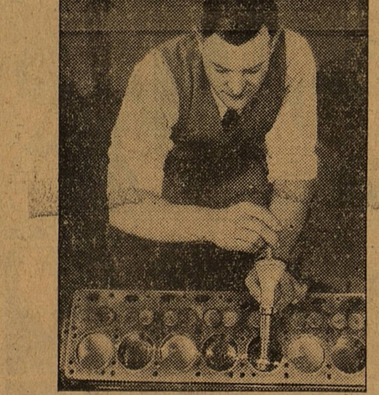
Measuring cylinder wear with a precision gauge—accurate to a hundred-thousandth of an inch!
