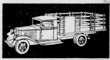
ECONOMICAL STAKE TRUCK-A rugged model that has broken records for low operating and upkeep costs. Special features include solidly-built platforn steel sign panels, hinged center stake section. 131" wheelbase. A buy of buys at ......
