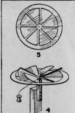
wide on the wide edge, and 1 1/2 inches wide on the narrow edge, and fasten them in the slots with nails. The hub block, with the blades in position, should next be pivoted to the end of the windmill shaft, a stick 16 inches long (Fig. 6). The end opposite to that to which the hub is pivoted is whittled round, and slotted with a saw to receive a tall (Fig. 8).
