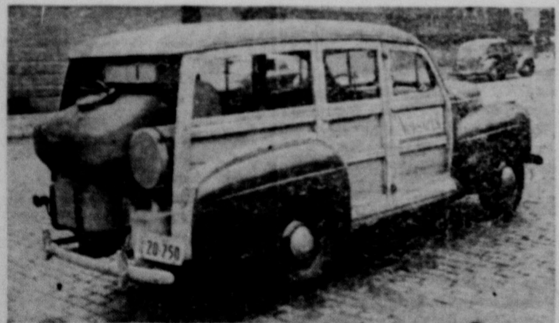
This is the small station wagon equipped with a gasogene that made the 800 mile experimental run from Kalamazoo, Mich., to New York city. The trip was a rigorous test for the efficiency of gas fuel, for the route led over the steep grades of the Allegheny mountains.
