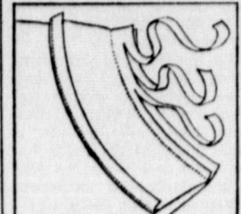
Seam edges are blended unevenly. Facing edge is always narrower than garment edge.
