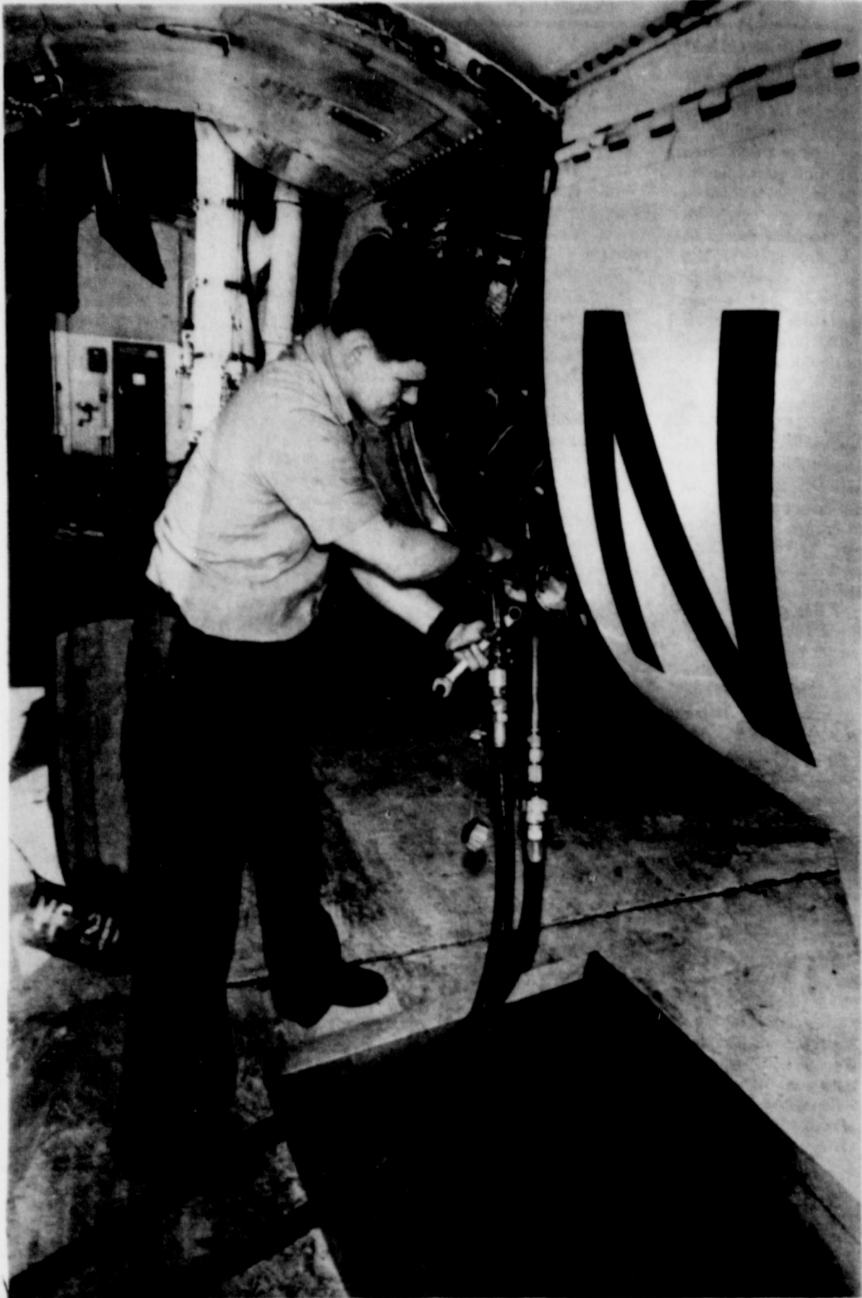
PETTY OFFICER THIRD class John Curry attaches a hydraulic fluid line to an F-14's hydraulic pump.
