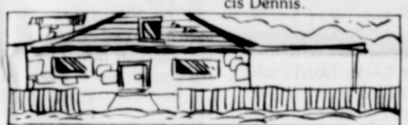
A house with small doors and windows is more energy-efficient than a structure with large window and door areas.
