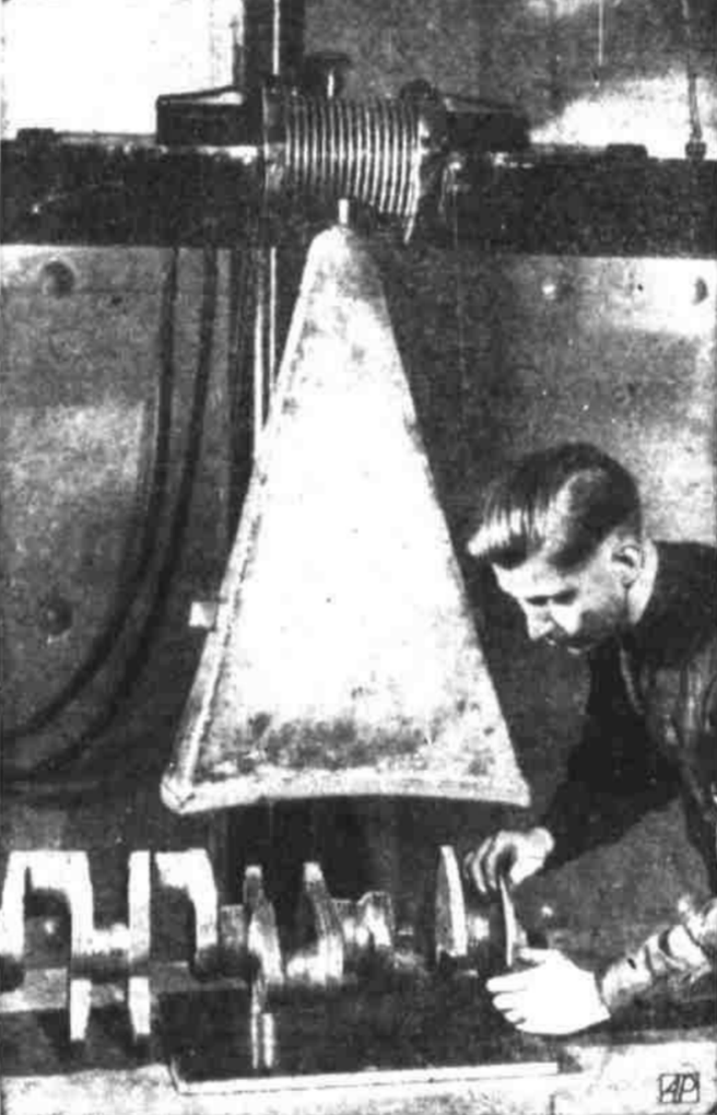
INSIDE DOPE ON CRANKSHAFT—Despite hesitancy of Henry Ford to build Rolls-Royce plane motors for Britain, workmen at Ford plant in Detroit speed up plans for mass production, even making X-rays of crankshafts (as above) and other machine parts. Ford has repeatedly said that he will make airplanes on a mass production basis only for the U. S. defense.
